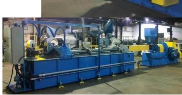
Flow molding is the process of extruding melted plastic directly from the plastic extruder into a mold of the shape required.
